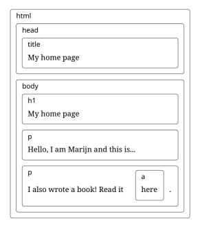
The data structure the browser uses to represent the document follows this shape. For each box, there is an object, which we can interact with to find out things such as what HTML tag it represents and which boxes and text it contains. This representation is called the *Document Object Model*, or *DOM* for short.
